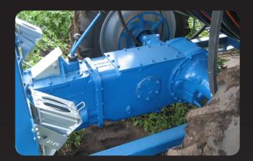
Reliable gearbox Note the reliable 6-speed MF 35 gearbox on which the FM 2500 machine is built.
