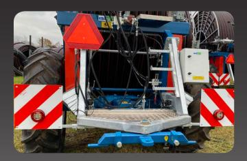
Traffic lights are standard All Fasterholt machines are today, as standard, equipped with traffic lights. Reflectors are optional equipment.
