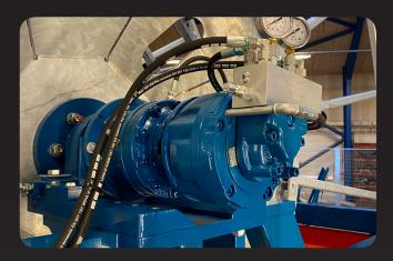
Hydraulic pull The hydraulic pull for winding up the hose ensures that it is always optimally positioned.
