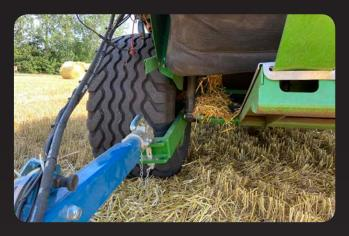
Durable ball-pull for easy connection and disconnection. Ensures stabile and steady drive of the wagon during work and transportation.
