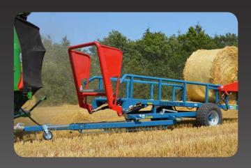
Strong loading platform with possibility of mounting an extra crossbow to adjusting the bale size.
