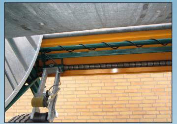
The worm axle is placed behind the front hose guide. This is supplied with an easy changeable guider in order to prevent the worm axle from wearing out. The hose guide is directly connected to the 3 stop safety system though the worm axle.
