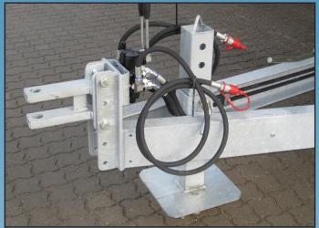
This machine is equipped with fork drawbar, but it can also be mounted with hitch eye pull. Notice the control valve for the hydraulic turning disc, support legs and gun wagon lift.
