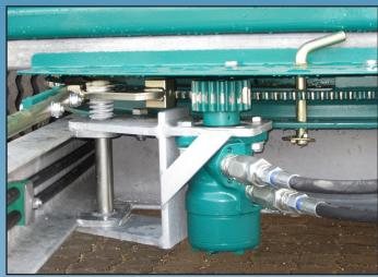
The hydraulic turning disc can be mounted as extra equipment. An oil motor provides secure and stable turning of the machine. A separate lock prevent unnecessary turning of the machine. The hydraulic hoses are hidden into the chassis, and the valve to both turning disc and support legs are placed on the chassis.
