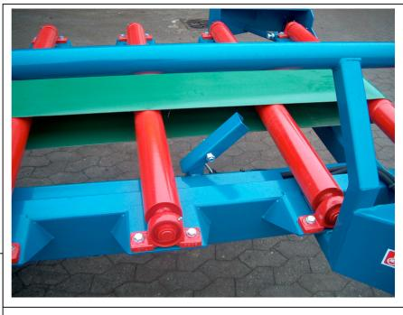
Balle switch is standard equipment on all types. Belt rollers are mounted in sealed bearings with lubricated bearing houses. QB-3 wagons is delivered with manual side sliding fixings for the wheel system's control cylinder. This must be moved laterally on road transportation.
