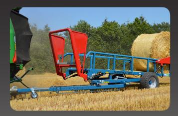
Strong loading platform with possibility of mounting an extra crossbow to adjusting the bale size.
