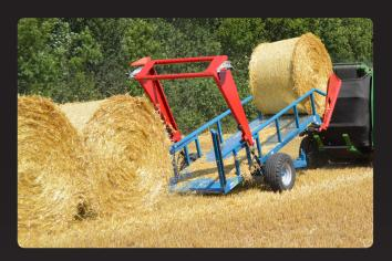
Hardwearing unloading gate with double active cylinders. Equipped with statutory light and marking devise and reflector.
